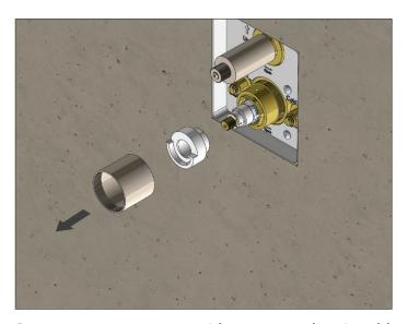
Remove temperature cartridge cover and anti-scald ring
