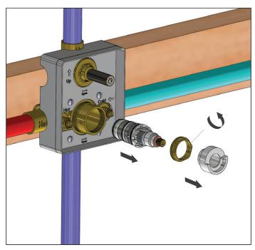
Remove anti-scald platic ring and loosen brass retaining nut. Then pull out cartridge.
