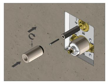
Insert extended black connecter and diverter connector
