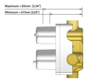
The distance between back of the valve to the finished tile surface should be between 2.63" and 3.34" inches.
