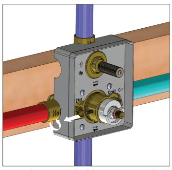
Remove hex nut on side of thermostatic cartridge.
