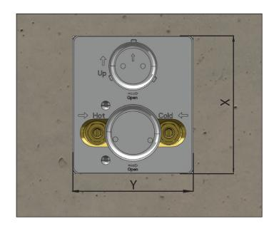
Isenberg's TVL valves comes with a black pre-attached mud-guard. This mud-guard is not to be removed or discarded. Its purpose is to guide the installation professional on the proper cut-out dimensions of the drywall.
