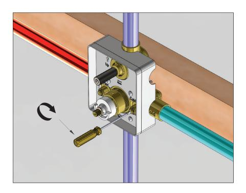
Turn Clock-wise 7 times to stop water flow.
